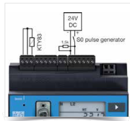
Fig.: Example temperature input (KTY83) and S0 pulse transducer
