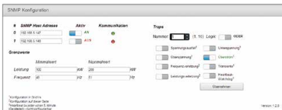
Fig.: Configuration page on an UMG without RCM functionality
